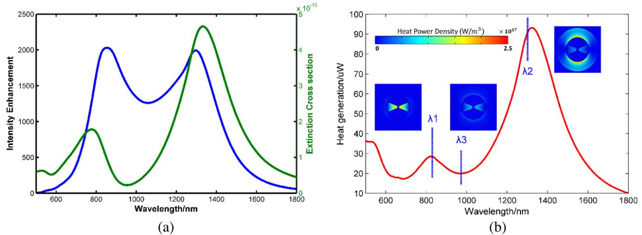
**Figure 4.** (a) Field intensity enhancement spectra (blue) and extinction cross section (green) of the structure. (b) Calculated spectra of the heat generation in antennas immersed in water. The three insets represent the heat power density at  $\lambda_1$ ,  $\lambda_2$  and  $\lambda_3$ .
