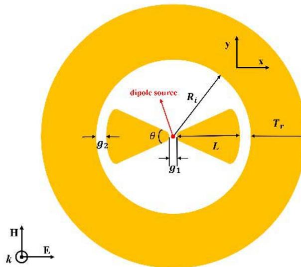
**Figure 1.** Top view of the plasmonic nanoantenna with broadband near field enhancement. It consists of a gold nanoring and a bowtie antenna at the center (BCR). The whole structure is immersed in water.
